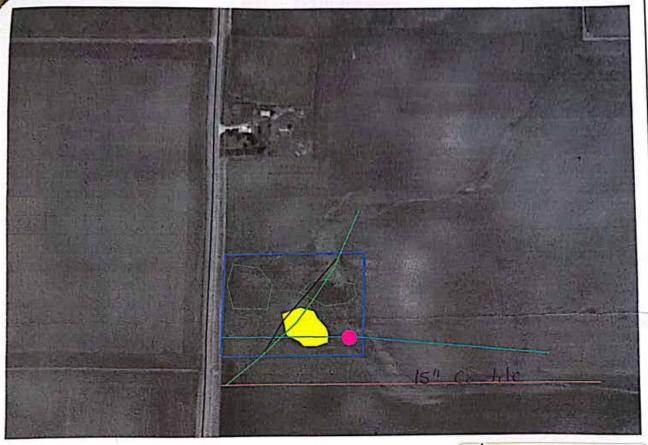
Replace 6" tile running through pond with 8" non-perforated tile. Remove at least 10' of the 6" at the hook-ups. Block 5" tile if it does not serve other areas.
